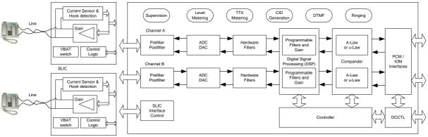
Figure 4 Functional overview of a two channel version of the example system
