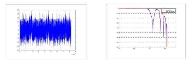
Figure 6 Time domain result (voltage over calculation points with 1/32MHz time distance) and FFT post-processing compared with a MATLAB frequency domain (ac) estimation (dB over frequency in Hz) for a decimation path (receive path)
