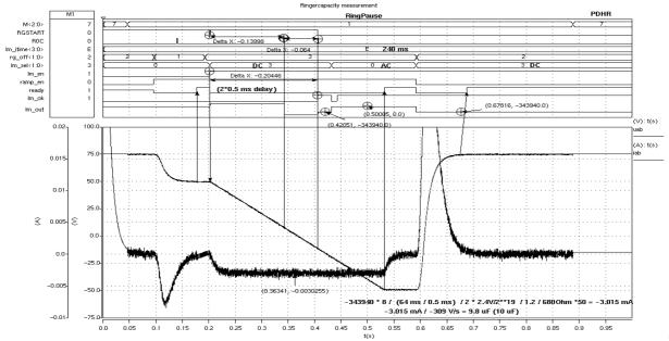
Figure 7 Example simulation of ringer capacity measurement
