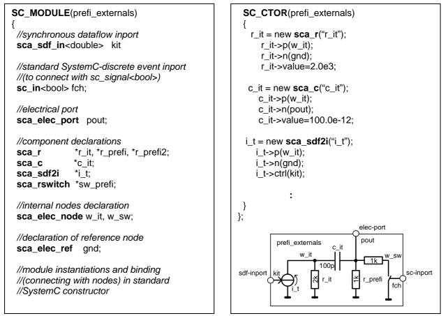
Figure 3 Hierarchical description of a conservative linear net
