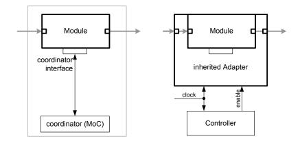
Figure 4: Refinement of interfaces by an inherited adapter class that uses the coordinator interface.
