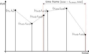
Figure 6: Abstract representation in polymorphic signal class by a queue of events (value, time).
