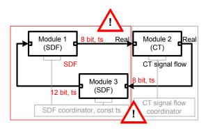
Figure 3: Computation-accurate model with inconsistencies due to refinement steps.
