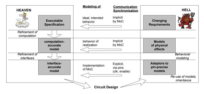
Figure 1: Refinement of signal processing applications to mixed-signal circuits with HEAVEN/HELL.
