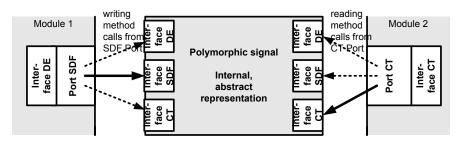
Figure 5: Implementation of polymorphic signals in SystemC-AMS.
