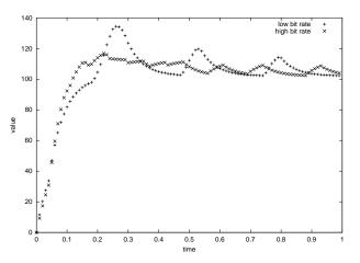
Figure 8: Output of PWM driver with different sample frequencies.
