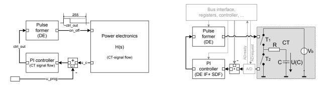
Figure 7: PWM driver: Executable specification (left), and after refinement (right).
